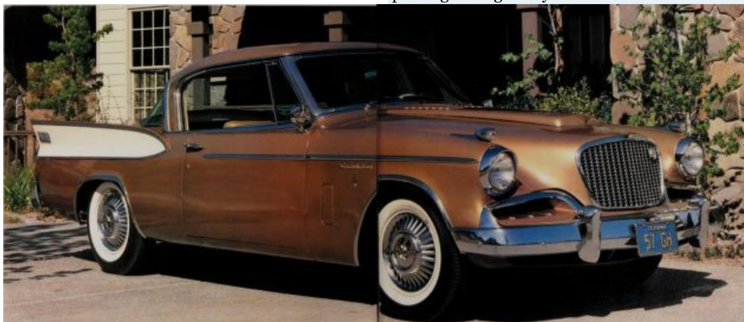
Wilder concave metal fins marked the '57 Golden Hawk, which handled much better than its '56 predecessor thanks to adoption of a lighter, supercharged Studebaker 289 V-8 in place of the heavy 352 Packard engine
