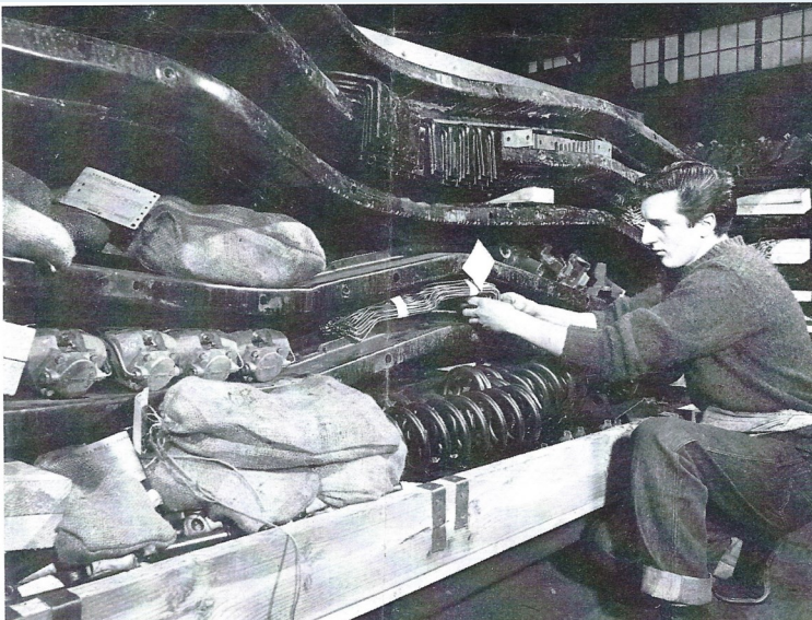
As much space as possible is being used here by packing between frames, such items as springs, tubing, hubs and drums, bags of components.
