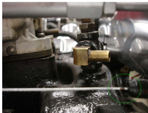
Position of TV Cable at full throttle (green circle) moves less than 1/2"
