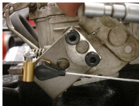
Position of TV cable at idle (see green circle)
