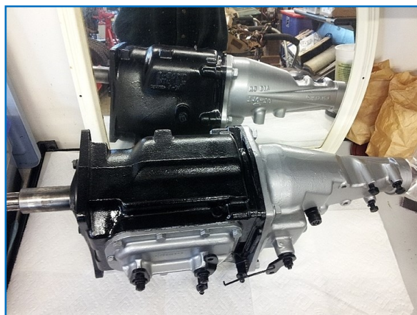
The completed rebuilt T10 4 speed transmission
